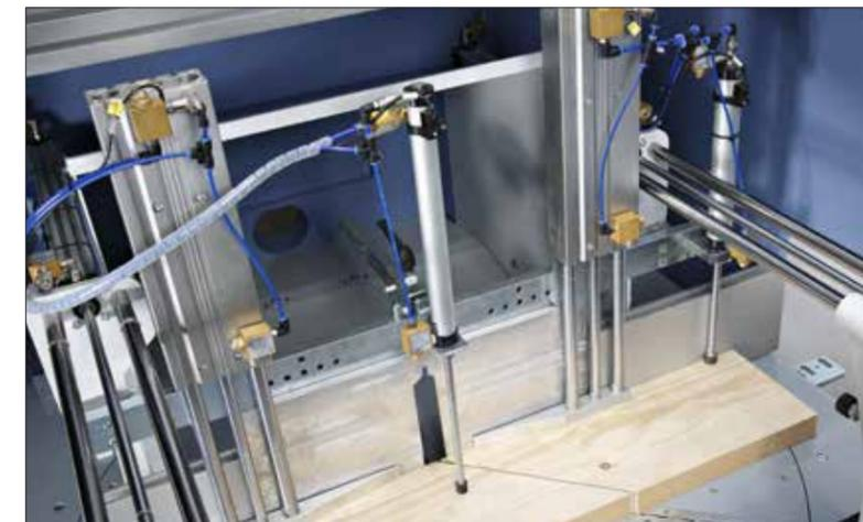
Trap door for expelling trimmed material from headpiece and scraps from straight cut tailpiece (closed)
